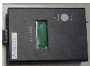
Figure 1-4 Ez-ISP (VDD supplied Standalone type ISP)
