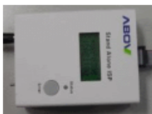
Figure 1-3 StandAlone ISP (VDD power is not supplied)
