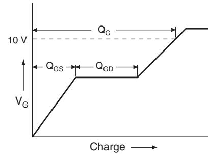
**Fig. 13a - Basic Gate Charge Waveform**
