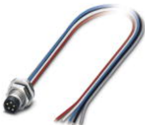
Bus system flush-type plug-in connector, plug, DeviceNet, 5-pos., M8, front/screw mounting with M10 fastening thread, with 0.5 m TPE litz wire, 5 x 0.25 mm²
