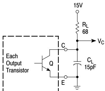
Figure 12. Common-Emitter Configuration
