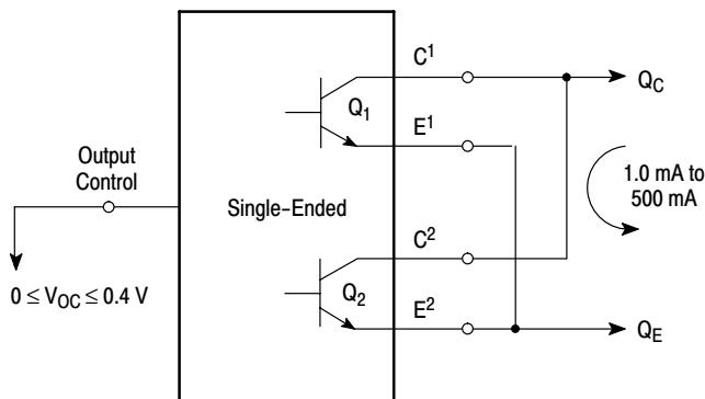
Figure 17. Output Connections for Single-Ended and Push-Pull Configurations
