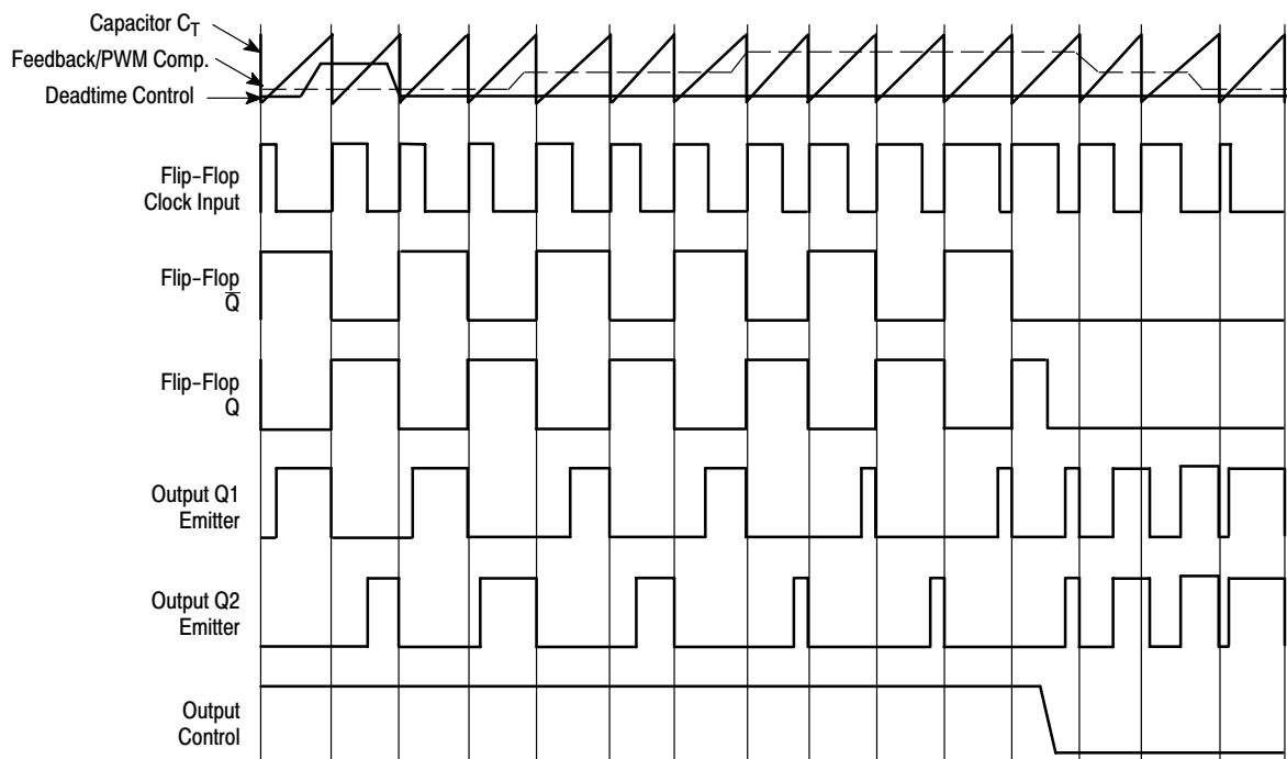
**Figure 2. Timing Diagram**
