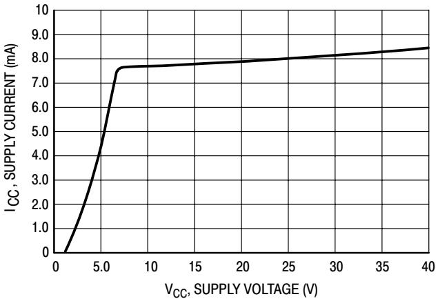
**Figure 9. Standby Supply Current versus Supply Voltage**
