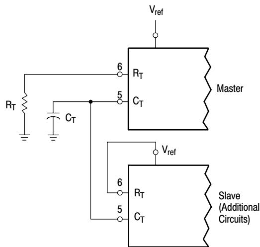
**Figure 18. Slaving Two or More Control Circuits**
