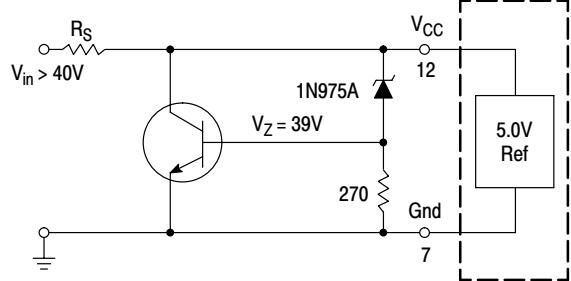
**Figure 19. Operation with  $V_{in} > 40$  V Using External Zener**
