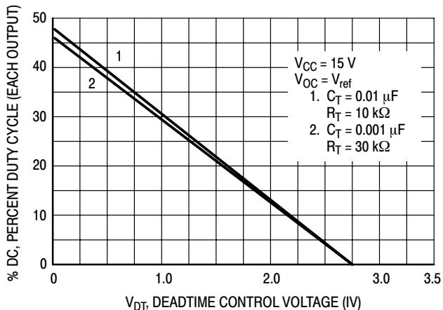
**Figure 6. Percent Duty Cycle versus Deadtime Control Voltage**
