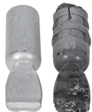
Uncrimped Good Contact
