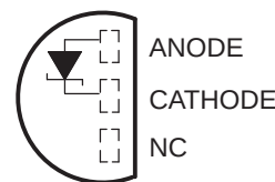
LP (TO-92/TO-226) PACKAGE (TOP VIEW)
