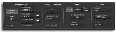
Spectrum analyzer style controls simplify waveform analysis in the frequency domain.
