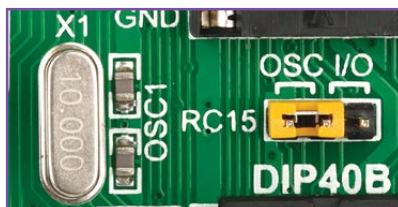
Figure 4-7: RC15 connected to X1 quartz-crystal
