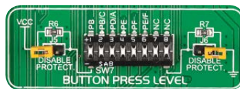
Figure 10-6: Button press level DIP switch (tri-state)
