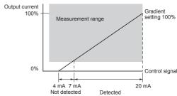
When the power regulator's gradient settings are changed, the operation gate current level is set so that the output current is within the measurement range. (In the following diagram, 14 mA is set.)
