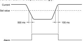
Transistor output models: ALM indicator lit, ALM transistor output Relay output models: ALM indicator lit, OR of all detection status output
