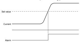
Transistor output models: ALM indicator lit, ALM transistor output Relay output models: ALM indicator lit, OR of all detection status output
