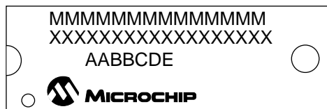
40-Lead CERDIP Windowed
