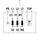
Note: Direction of rotation changes when two phases are reversed
