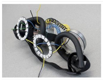
If using the "bring your own goggles" method, things may be a lot more complex...for example, these goggles have wires passing in and out through side perforations, so it's not possible to build and test the whole circuit separately first...it must be built around the goggles and is later folded into place. This is tricky!
