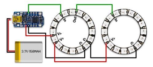
This diagram uses the original Trinket but you can also use the Trinket M0 with the exact same wiring!
