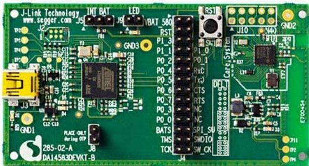
This Basic development kit gives you all flexibility to develop with confidence. All of the DA14583's I/Os are available and mapped on to expansion connectors. A debugger is provided on the PCB which in combination with SmartSnippets™, Dialog's complete software environment, enables you to program and test your Bluetooth Smart application.
