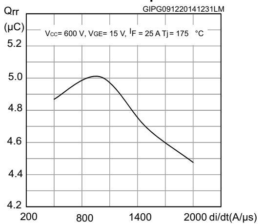
**Figure 26. Reverse recovery energy vs. diode current slope**
