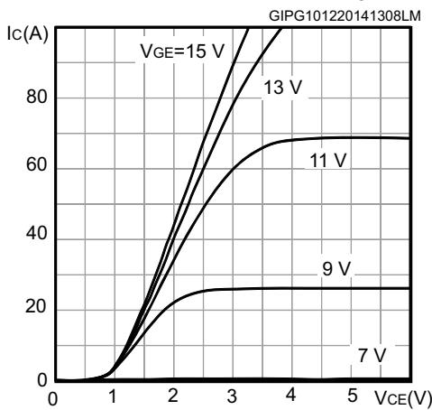
**Figure 5. Output characteristics ( $T_J = 175 \text{ }^\circ\text{C}$ )**
