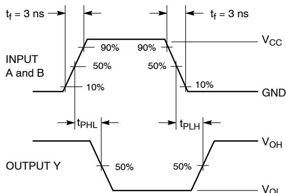
**Figure 3. Switching Waveform**
