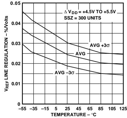
Figure 25. Reference Line Regulation vs.
