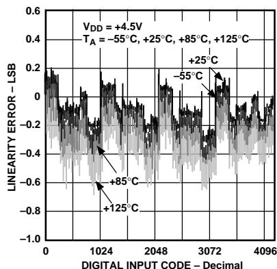
Figure 1. Linearity Error vs. Digital Code & Temperature
