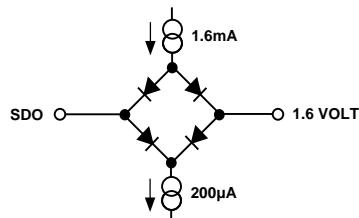
Figure 3. AC Timing SDO Pin Load Circuit
