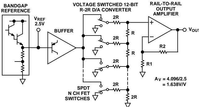
Figure 4. Equivalent AD8522 Schematic of Analog Portion
