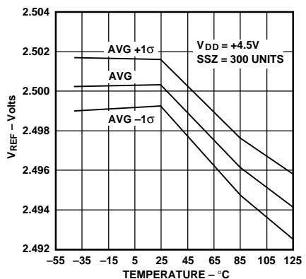
Figure 23. Reference Voltage vs.
