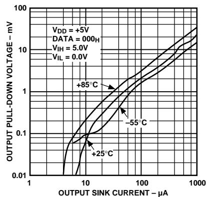
Figure 8. Pull-Down Voltage vs. Output Sink Current Capability
