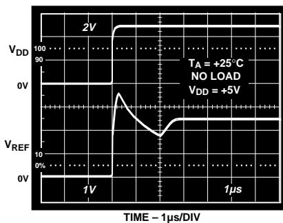
Figure 21. Reference Startup vs.
