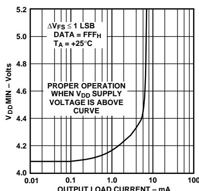
Figure 7. Minimum Supply Voltage vs. Load Current
