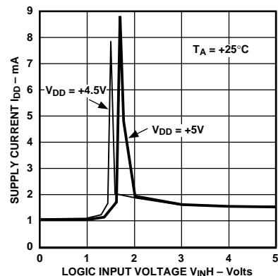
Figure 11. Supply Current vs. Logic Input Voltage
