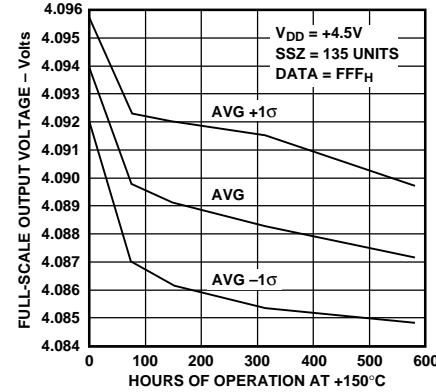
Figure 19. Long Term Drift Accelerated by Burn-In
