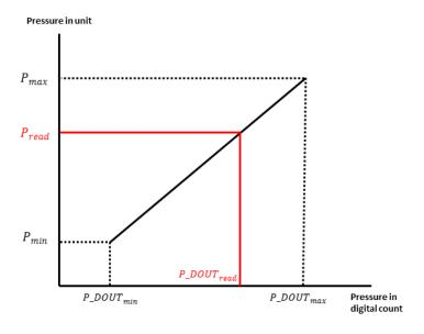
For example, the  $P_{min}$  and  $P_{max}$  for the sensor are specified as -0.3 and +0.3 psi. The  $DOUT_{min}$  and  $DOUT_{max}$  are -26214 and +26214. So,
