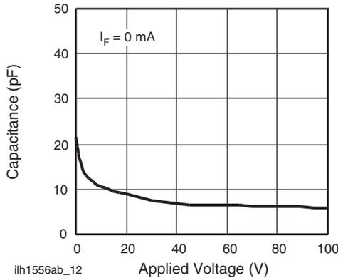
Fig. 13 - Switch Capacitance vs. Applied Voltage
