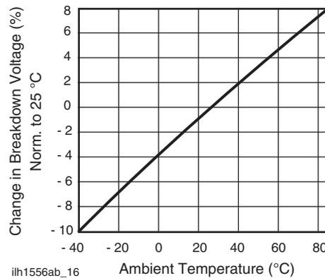
Fig. 17 - Switch Breakdown Voltage vs. Temperature
