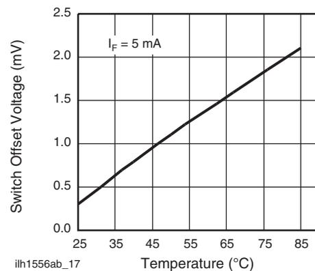
Fig. 18 - Switch Offset Voltage vs. Temperature
