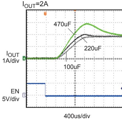
1Ω Load Connected to Enabled Device
