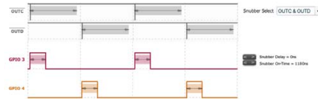
Figure 46. Active Clamp Snubber Configured on OUTx Signals
