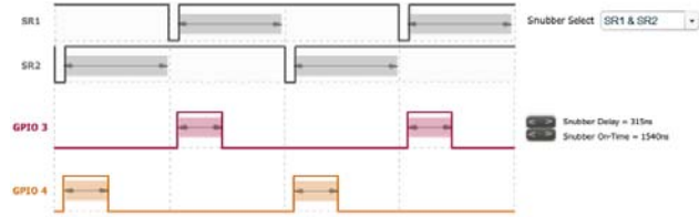
Figure 45. Active Clamp Snubber Configured on SRx Signals
