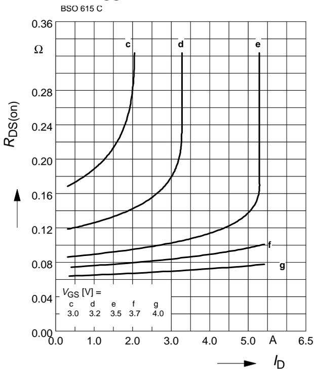
**Typ. drain-source-on-resistance (P-Ch.)**
