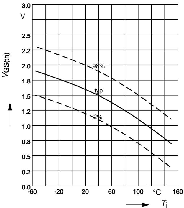
**Gate threshold voltage (P-Ch.)**
