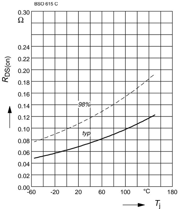
**Drain-source on-resistance (P-Ch.)**
