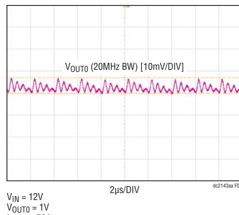
Figure 7. Output Voltage Ripple
