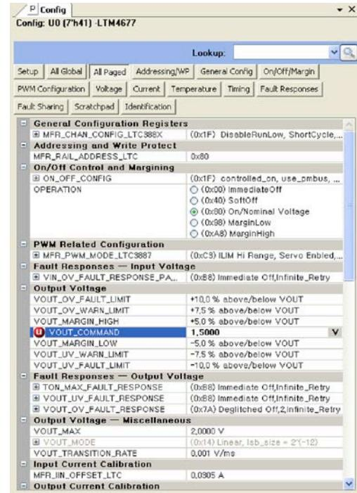
Then, click the W (PC to RAM) icon to write these register values to the LTM4677. After finishing this step, you will see the output voltage will change to 1.5V.
