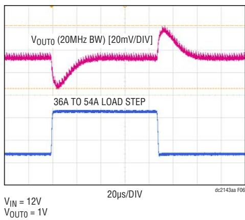
Figure 6. Output Voltage  $V_{OUT0}$  vs Load Current
