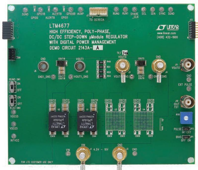
Figure 1. 2x LTM4677; 72A DC2143A-A Demo Circuit
