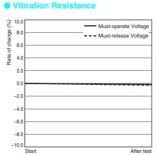
Characteristics were measured after applying vibration at a frequency of 5 to 200 to 5 Hz, acceleration of 44.1 m/s<sup>2</sup> to the test piece (not energized) for 2 hours each in 3 directions. The percentage rate of change is the average value for all of the samples.
