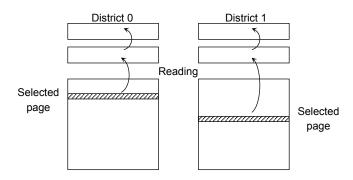
The data transfer operation from the cell array to the Data Cache via Page Buffer starts on the rising edge of  $\overline{\text{WE}}$  in the 30h command input cycle (after the 2 Districts address information has been latched). The device will be in the Busy state during this transfer period.
