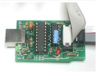
Plug in the two cables as shown, the red stripes on top and so that the cables don't bend over the plug (the case wont fit).
