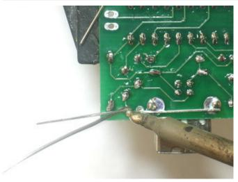
Solder and clip the two LEDs.
