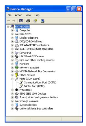
Under ports you'll see a list of COM ports. Both of the virtual ports we're making have to be between COM1 and COM9. Looks like only COM1 is being used.
