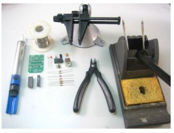
Get your tools ready! A board vise, soldering iron & solder, diagonal cutters, and a solder sucker (desoldering tool) if you have one.
