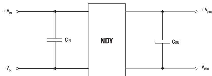
Recommended circuit for reduced ripple 3.3V output
