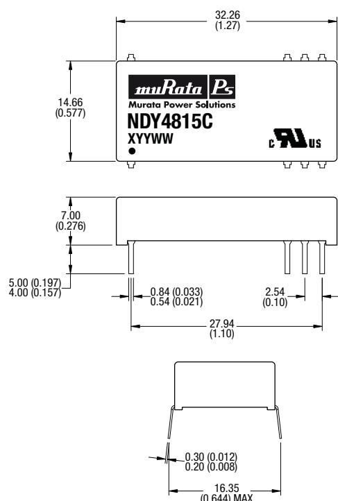
All dimensions in mm  $\pm 0.25$ mm (inches  $\pm 0.01$ ). All pins on a 2.54 (0.1) pitch and within  $\pm 0.25$  (0.01) of true position.
