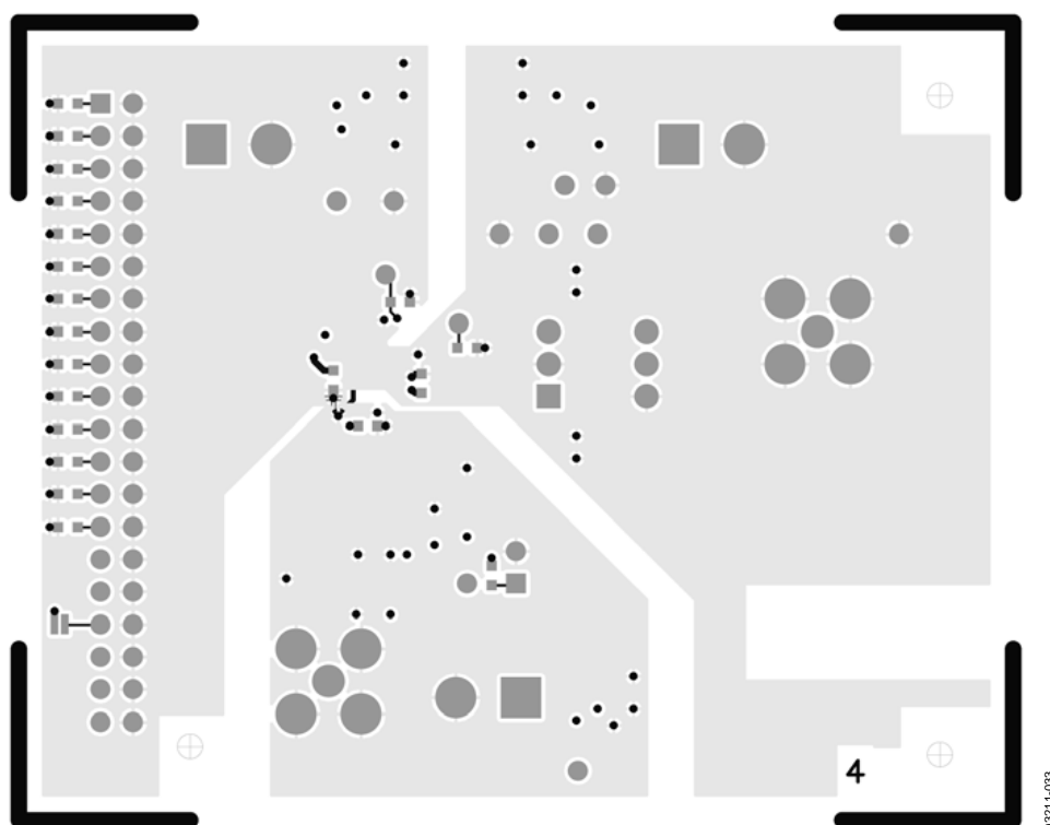
Figure 36. Evaluation Board Layout—Secondary Side
