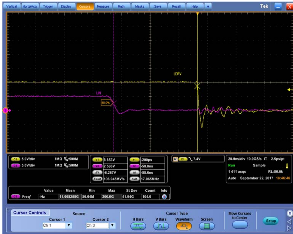
Figure 31. Low Side Turn-Off Propagation Delay (NCP51530A)
