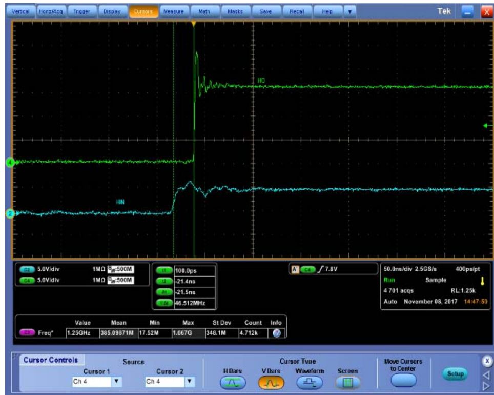
Figure 32. High Side Turn-Off Propagation Delay (NCP51530B)
