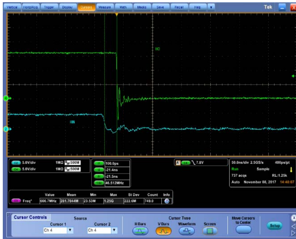
Figure 33. High Side Turn-Off Propagation Delay (NCP51530B)
