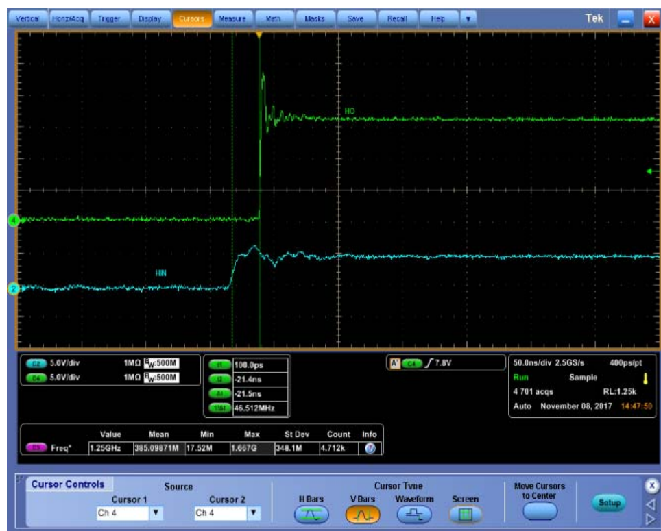
Figure 32. High Side Turn-Off Propagation Delay (NCP51530B)
