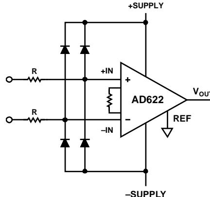
Figure 18. Diode Protection for Voltages Beyond Supply
