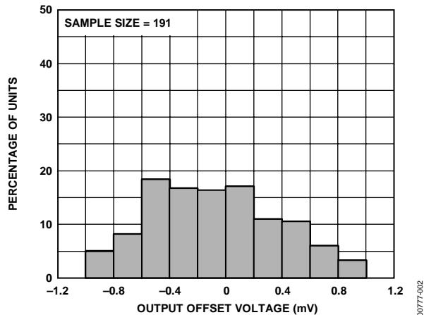
Figure 2. Typical Distribution of Output Offset Voltage
