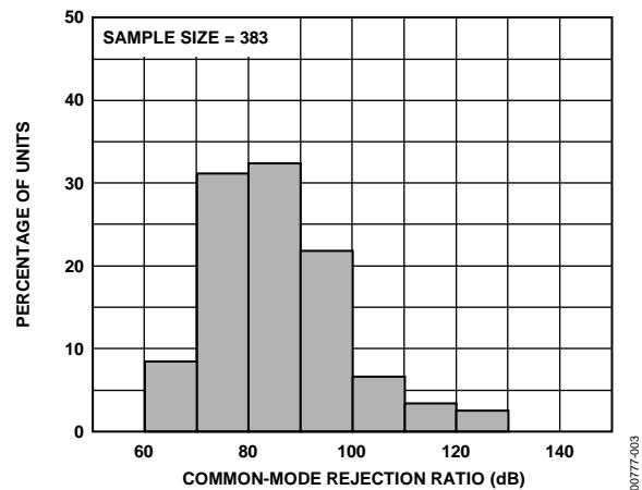
Figure 3. Typical Distribution of Common-Mode Rejection
