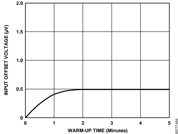
Figure 4. Change in Input Offset Voltage vs. Warm-Up Time
