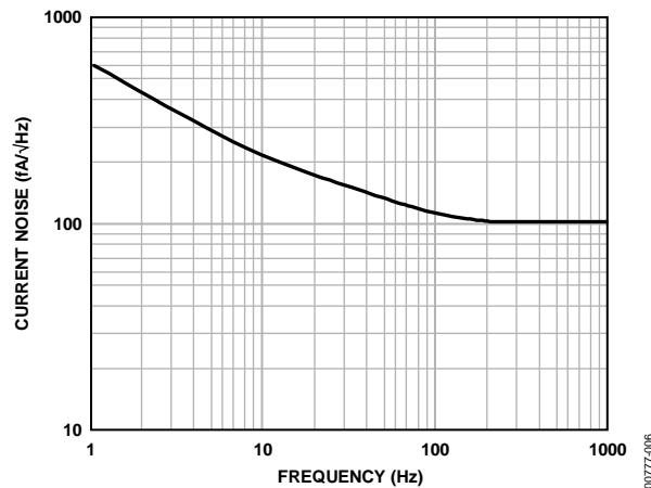
Figure 6. Current Noise Spectral Density vs. Frequency
