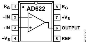
Figure 1. 8-Lead PDIP and 8-Lead SOIC\_N
