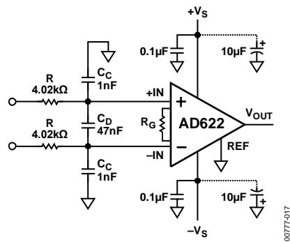
Figure 19. RFI Suppression Circuit for AD622 Series In-Amps
