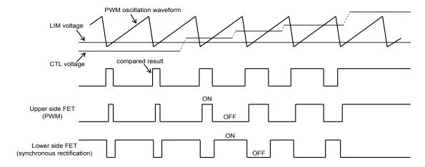
If a minus voltage is applied to the CTL pin, this pin current must be limited within 2mA by inserting the resistor of about  $200\Omega$ .
