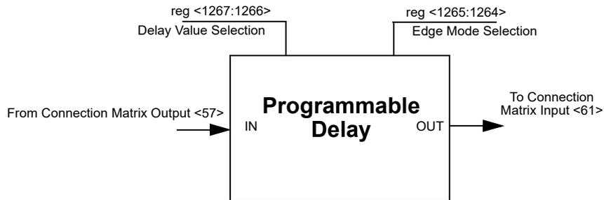
Figure 59. Programmable Delay
