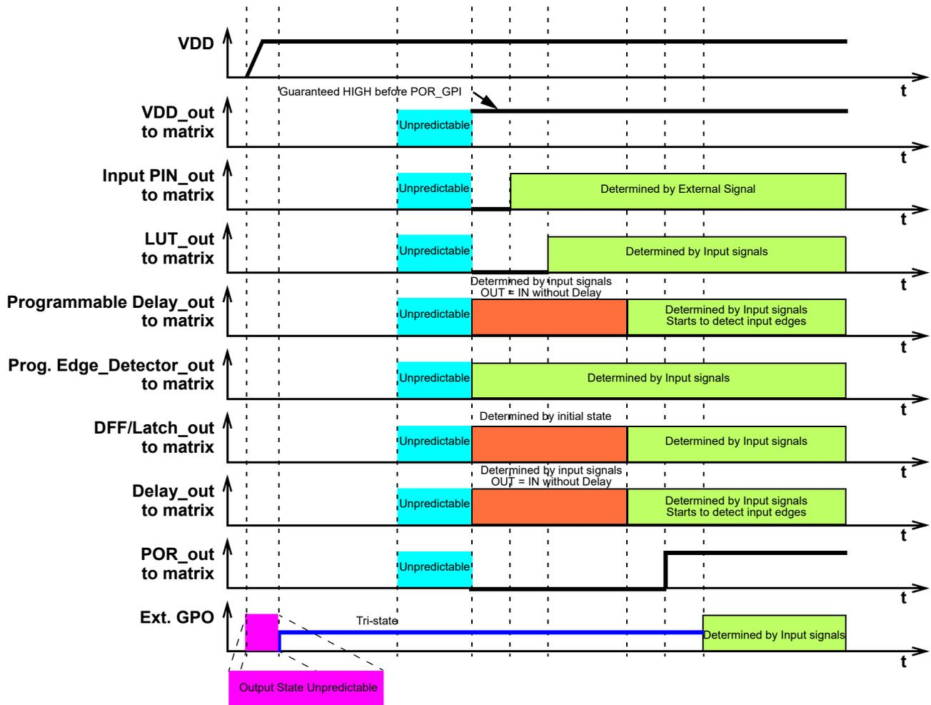
Figure 78. Internal Block States during POR sequence
