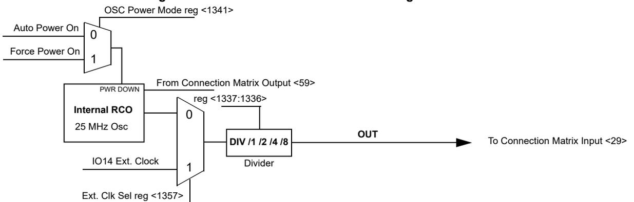
Figure 67. 25 MHz RC OSC Block Diagram
