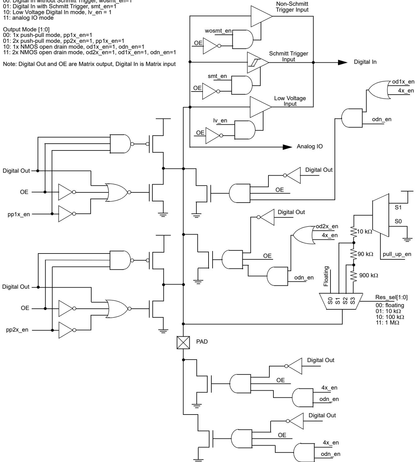
Figure 5. Matrix OE IO 4X Drive Structure Diagram
