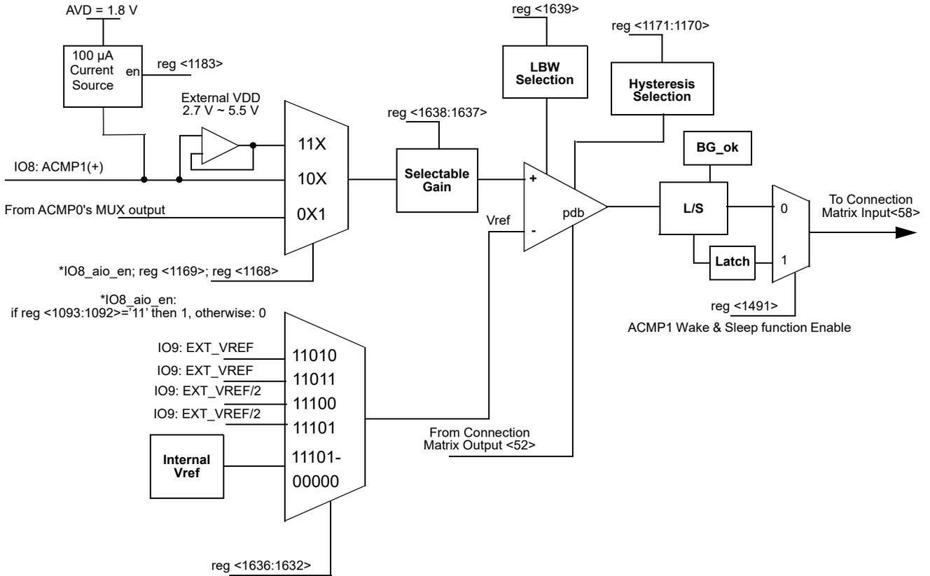
Note: when 100  $\mu$ A Current Source is enabled input voltage on IO8 should not exceed 1.8 V
