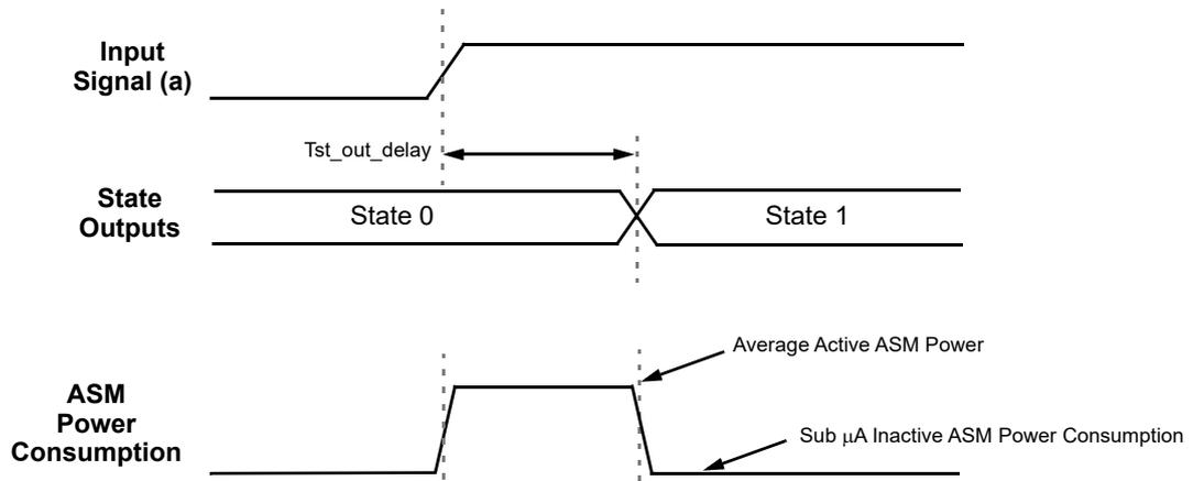
Figure 89. State Transition Timing and Power Consumption
