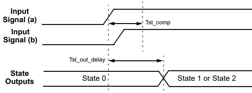
Figure 93. State Transition Timing - Competing Inputs Indeterminate
