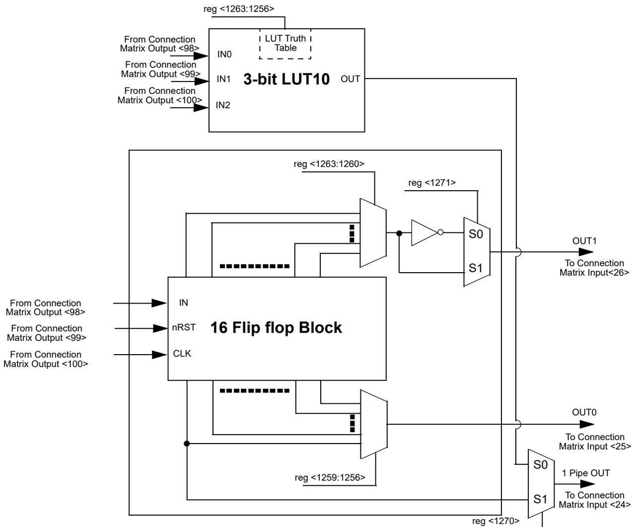
Figure 28. 3-bit LUT10 or Pipe Delay
