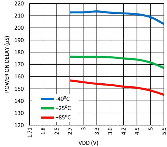
**Figure 52. Maximum Power On Delay vs. VDD, BG = 100 μs.**
