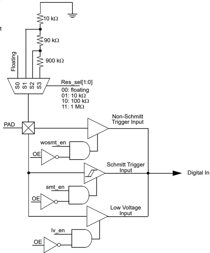
Figure 2. IO0 GPI Structure Diagram
