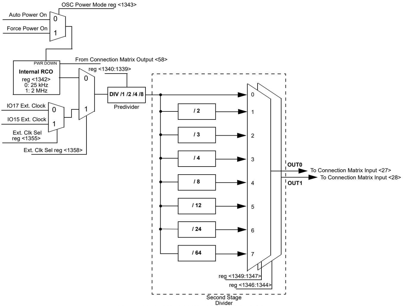
Figure 66. 25 kHz / 2 MHz RC OSC Block Diagram
