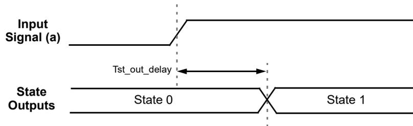
Figure 87. State Transition Timing
