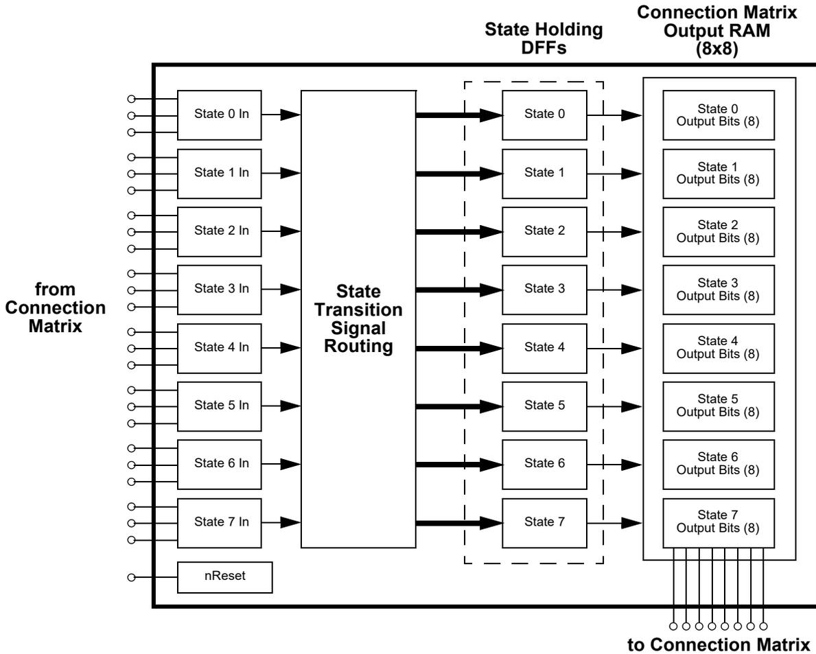
Figure 81. Asynchronous State Machine
