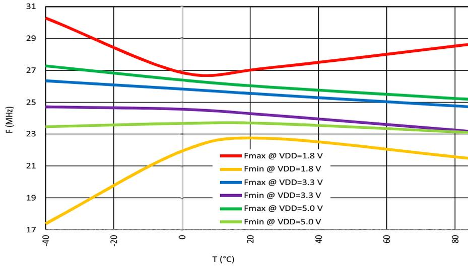
Figure 74. OSC1 (25 MHz) Frequency vs. Temperature
