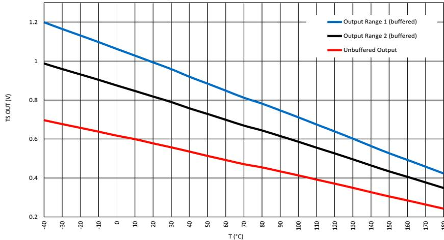
Figure 109. TS Output vs. Temperature, VDD = (1.71...5.5) V
