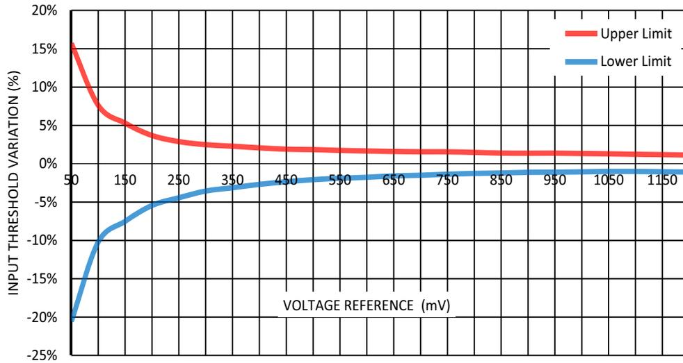
Figure 54. Typical Input Threshold Variation (including Vref variation, ACMP offset) vs. Voltage Reference at T = (-40.... +85)°C, LMB Mode - Disable, V<sub>hys</sub> = 0 mV.
