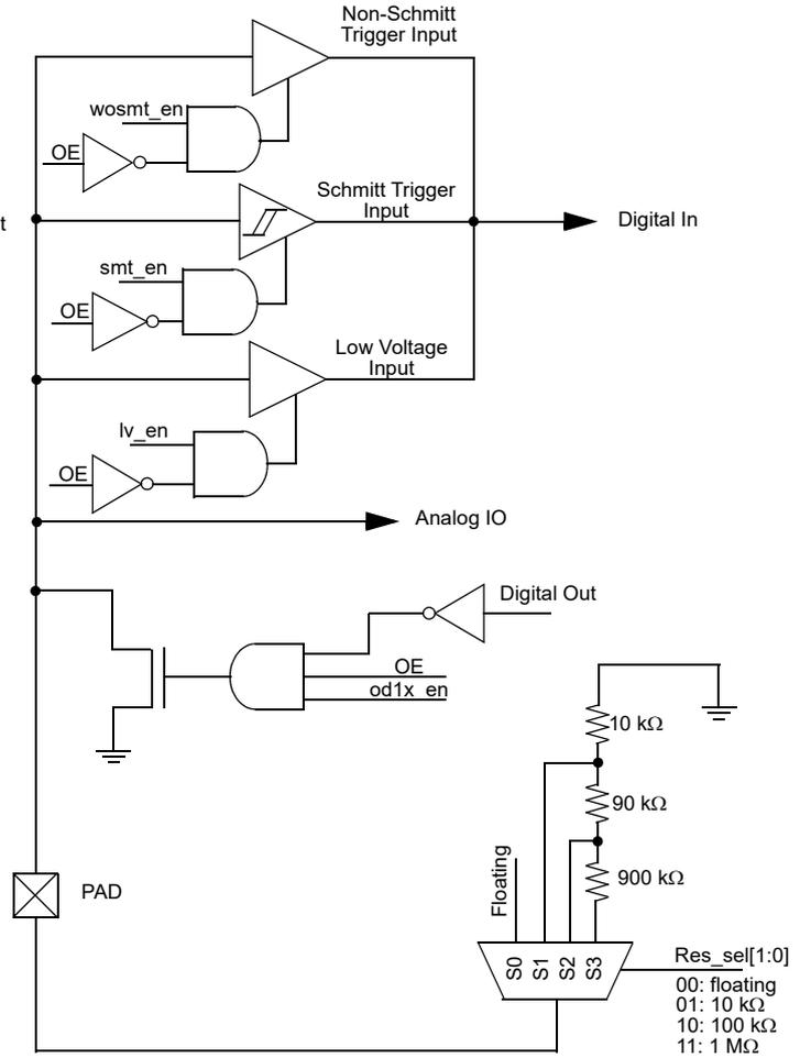
Figure 4. Matrix OE IO Structure Diagram
