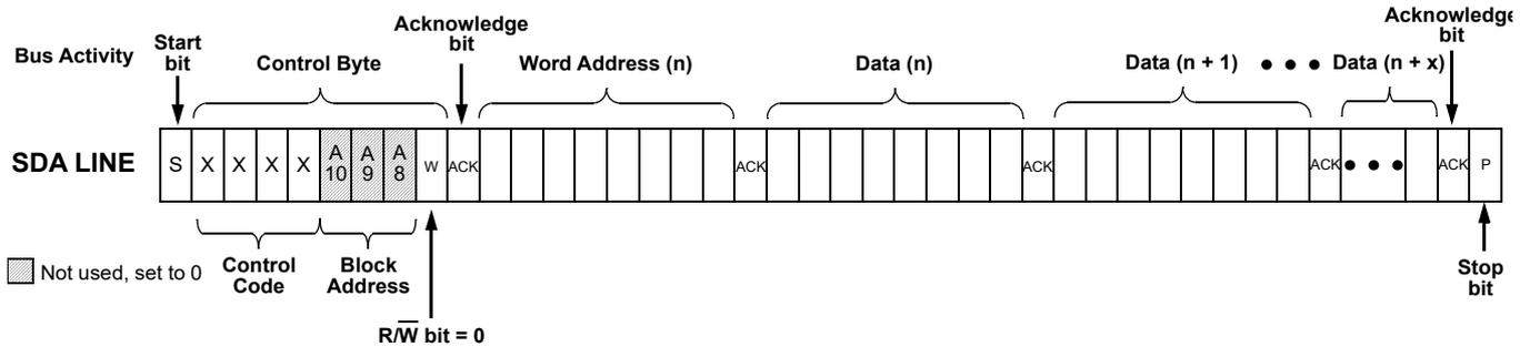
Figure 102. Sequential Write Command,  $\overline{R/W} = 0$
