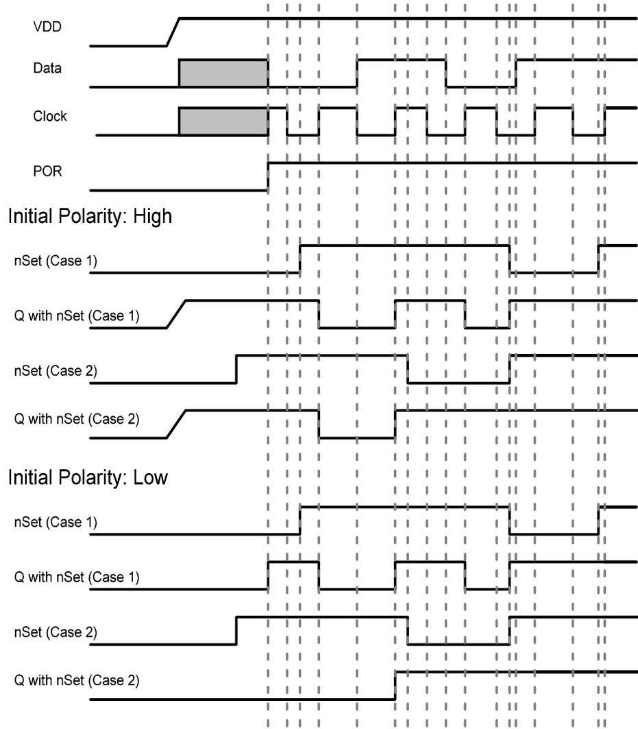
Figure 27. DFF Polarity Operations with nSet
