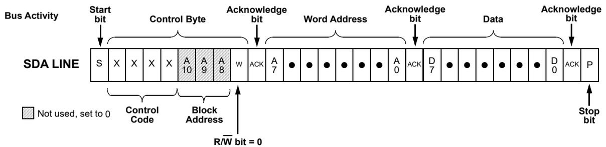
Figure 101. Byte Write Command, R/W = 0
