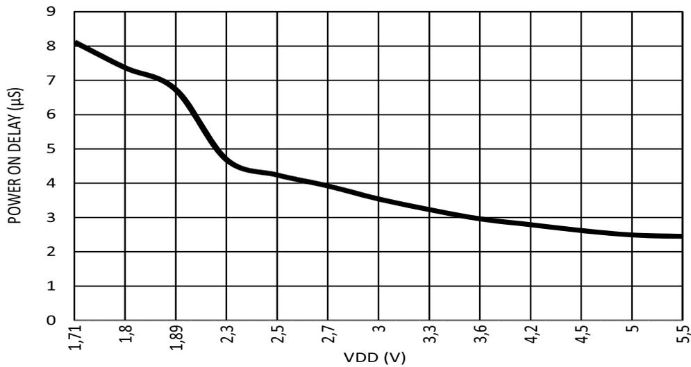
Figure 71. OSC1 (25 MHz) Maximum Power On Delay vs. VDD at room temperature
