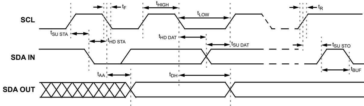
Figure 100. I<sup>2</sup>C General Timing Characteristics
