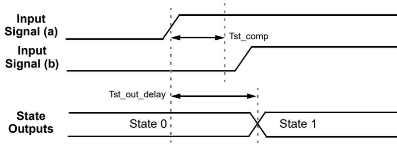
Figure 94. State Transition Timing - Competing Inputs Determinable
