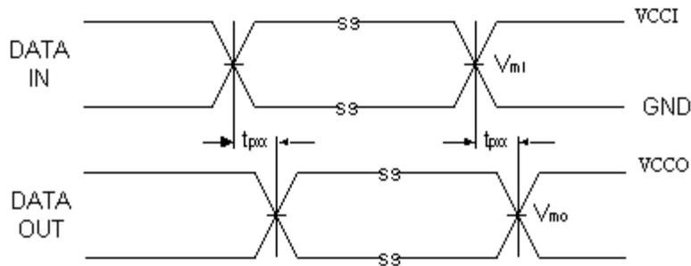
**Figure 5. Waveform for Inverting and Non-Inverting Functions**
