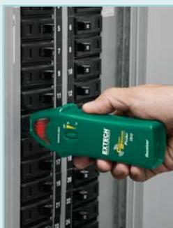
Adjustable sensitivity for pinpointing the correct breaker
