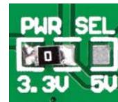
On-board **PWR SEL** zero-ohm resistor (SMD jumper) is used to determine whether 5V or 3.3V power supply is used. This resistor is provided in 3.3V position by default. In order to use SHT1x click with 5V development system, it is necessary to resolder this jumper to 5V position.
