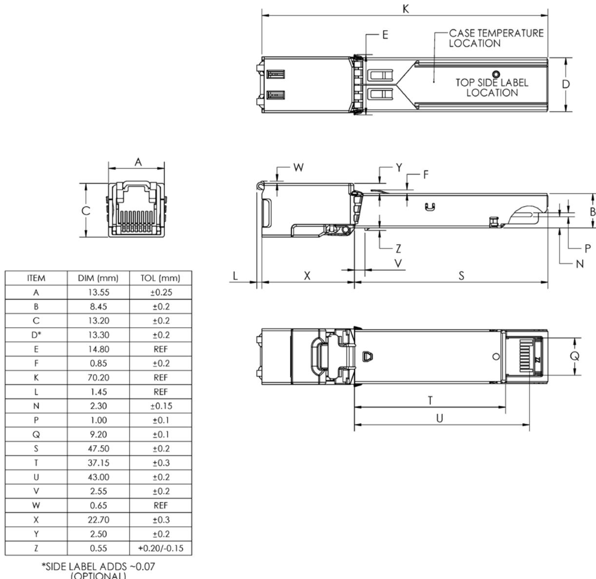
**Figure 2. FCLF8520P2BTL, FCLF8521P2BTL and FCLF8522P2BTL mechanical dimensions**
