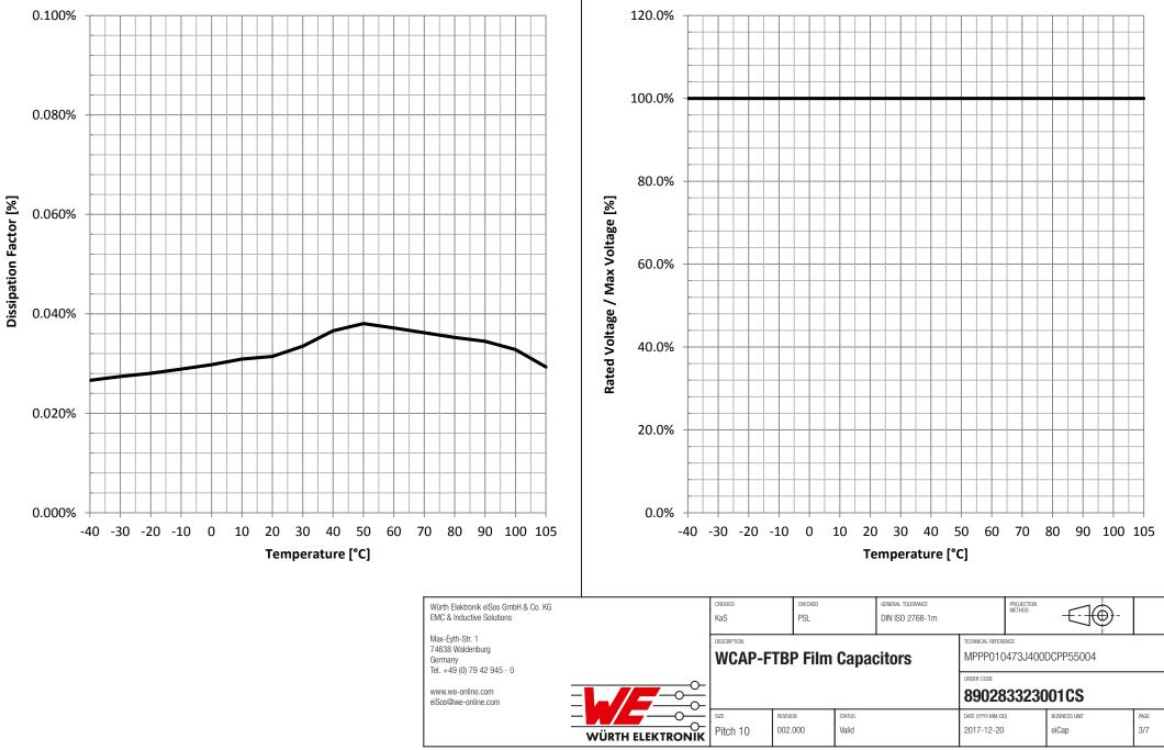
**Rated Voltage vs. Temperature:**
