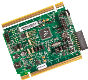
Figure 3: TWR-S08MM128 with Default Jumpers Used in Table 1
