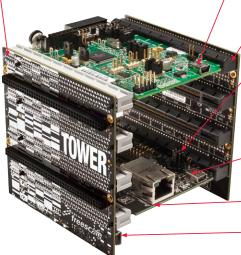
Figure 2: Tower System Assembled NOTE: Figure 2 is a Tower System without the optional MED-EKG assembly. For details on how to assemble the MED-EKG, please refer to Lab 1 on the DVD.
