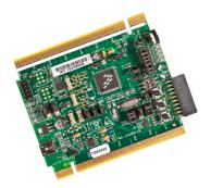
Figure 3: TWR-S08MM128 with Default Jumpers Used in Table 1
