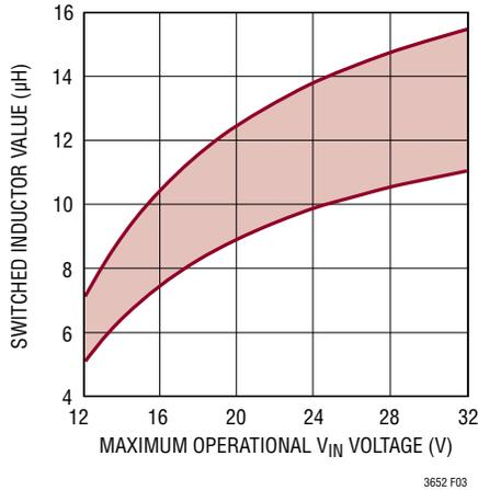
Figure 3. 7.2V at 1.5A Switched Inductor Values
