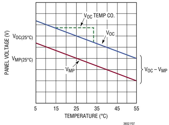
Figure 7. Temperature Characteristics for Solar Panel Output Voltage
