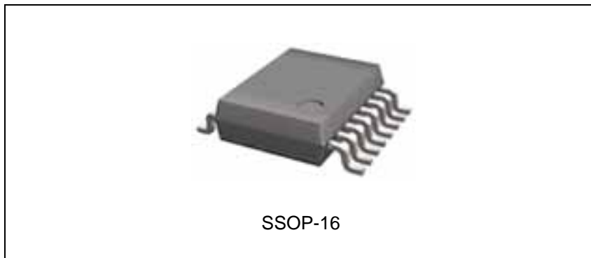
Figure 1. Package Type of AM4967
