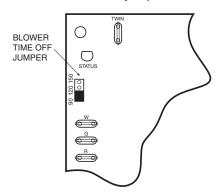
The control is factory set to give a (150) second blower off delay. See drawing below for the jumper position for all available settings:
