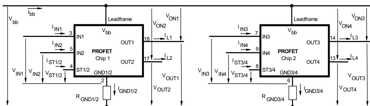
Leadframe ( $V_{bb}$ ) is connected to pin 1,10,11,12,15,16,19,20
