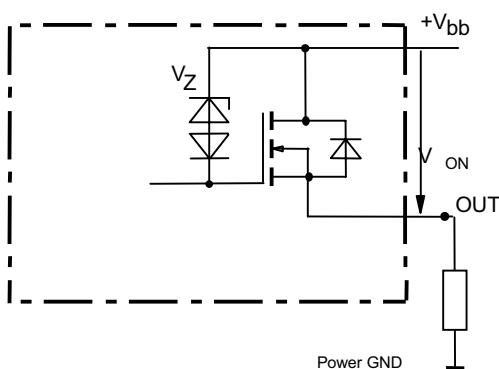
$V_{ON}$  clamped to  $V_{ON(CL)} = 47$  V typ.
