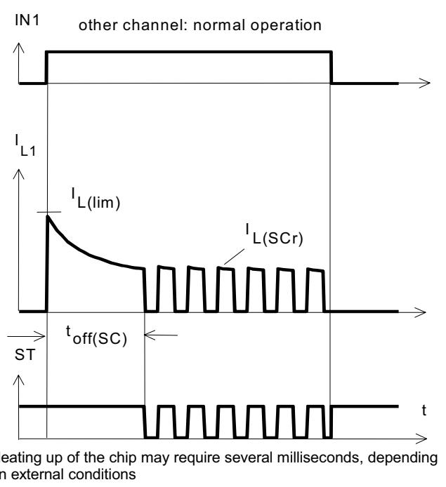
**Figure 3b:** Turn on into short circuit:
