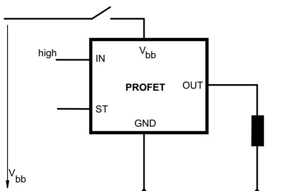
For inductive load currents up to the limits defined by  $Z_L$  (max. ratings and diagram on page 10) each switch is protected against loss of  $V_{bb}$ .
