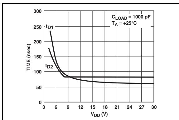
**FIGURE 2-4:**  $t_{D1}$  and  $t_{D2}$  Delay vs.  $V_{DD}$ .
