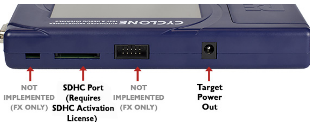
Figure 3-4: Cyclone LC Rear Side View
