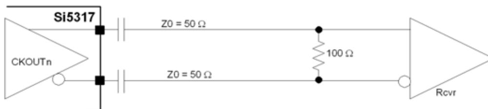
Figure 11. Typical Differential Output Circuit
