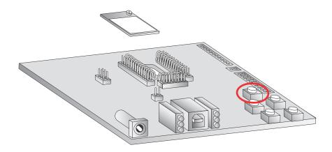
Pressing this button power cycles the module, but will not clear any changes written to the module. This is useful if you are having issues accessing the COM port. This will also reset any parameters that were changed but not written into memory.
