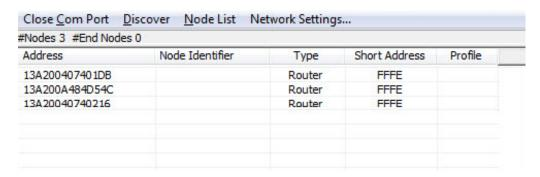
By selecting a particular node from the list, you can interact with it as if it were connected to the PC directly. Now you can Read, Write, and Restore parameters on the main X-CTU window, and those changes will occur over the air on the remote module selected in the Network window. Close the Network window when you have finished with remote configuration.
