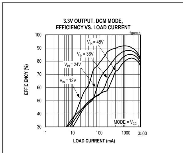
Figure 5. MAX17504 3.3V Output Efficiency (DCM Mode)
