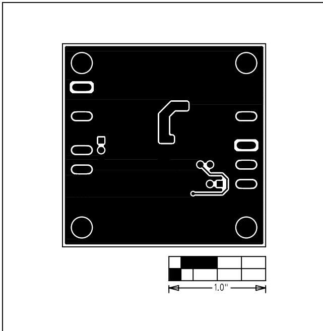
Figure 16. MAX17504 3.3V Output EV Kit PCB Layout—
