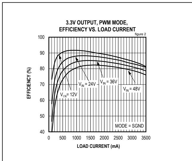
Figure 2. MAX17504 3.3V Output Efficiency (PWM Mode)
