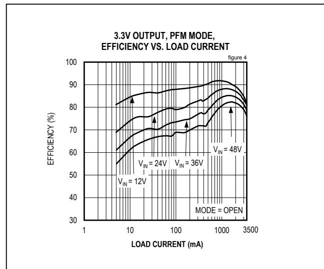
Figure 4. MAX17504 3.3V Output Efficiency (PFM Mode)
