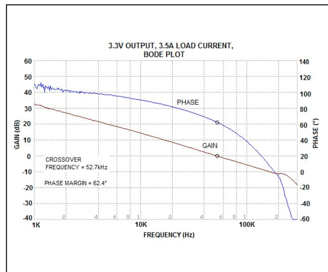
Figure 6. MAX17504 3.3V Output Full Load Bode Plot ( $V_{IN} = 24V$ )
