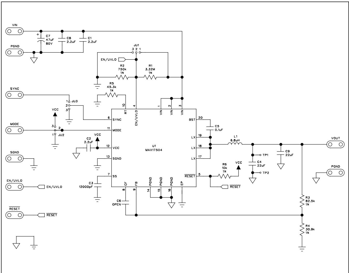
Figure 11. MAX17504 3.3V Output EV Kit Schematic
