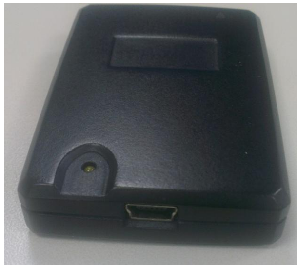
Figure 1-3: Rear panel showing the USB connector
