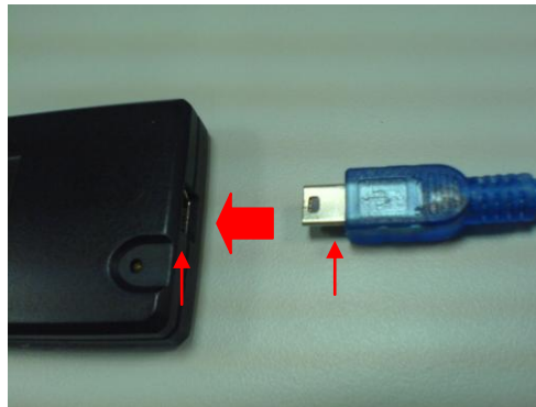
Figure 2-16: Connect the USB cable to the Logic Analyzer
