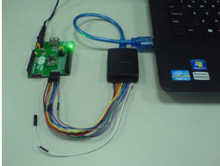
Figure 2-25: An Assembly of Laptop, Logic Analyzer, and DUT
